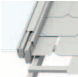
Model EDS Flashing for a single window. Available as standard in grey-painted aluminium. For flat roofing materials up to a thickness of 16 mm (2 x 8 mm).
